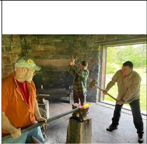
Fig. 6 NGM Blacksmiths Forging Lug Pole
