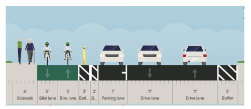
Parking Protected Cycle-Track with Sidewalk, Cross-Section (Image credit: Streetmix.net, TPD). See also — Segment B, Cross Section #1 earlier in this chapter.
