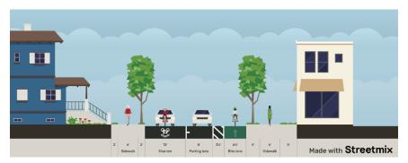
Contra-Flow Bike-Lane with On-Road Shared Lane Marking and Sidewalk, Cross-Section. (Image credit: Streetmix.net, TPD) See also — Segment D, Cross Sections #2 & #3, earlier in this chapter.
