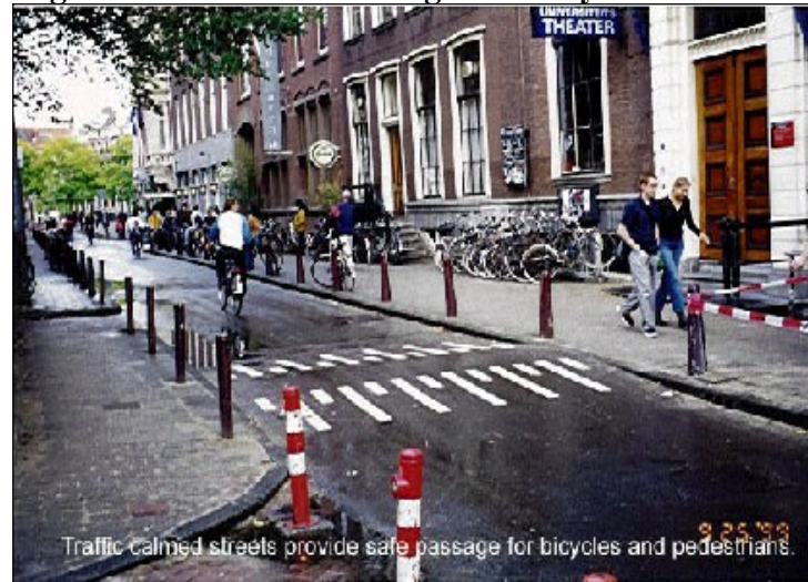
Figure 5-5: Traffic Calming for a Bicycle Boulevard
