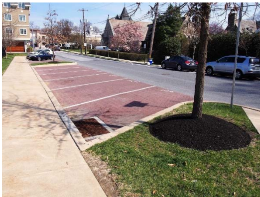
Figure 4-3: Front-in angle parking in Wayne along U.S. Route 30 and perpendicular streets makes it difficult and dangerous for cars to leave a parking spot.
