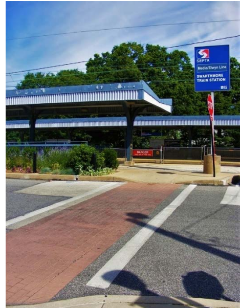
Figure 4-11: Brick paver crosswalks, such as the one that guides pedestrian access to Swarthmore Station, are more visible to drivers and can help make crosswalks safer.
