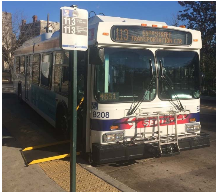
Figure 4-14: The ADA lift on this bus provides access for passengers using wheelchairs, and the yellow detectable warning strip at the edge of the boarding area helps vision-impaired passengers board safely.
